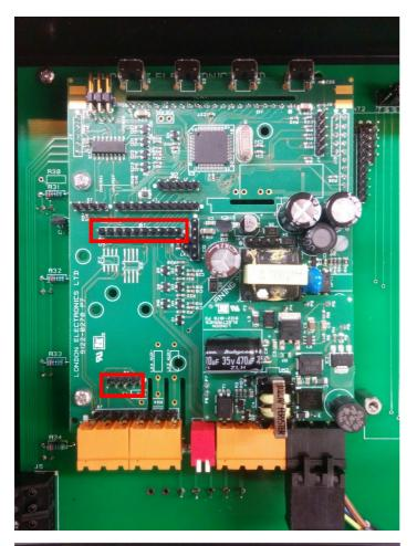
The Handling board attaches to the Fusion Display main card using the highlighted header pins.
