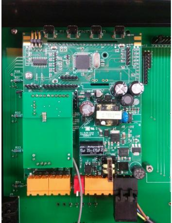
Left. Handling Board attached to Fusion Display main card.
