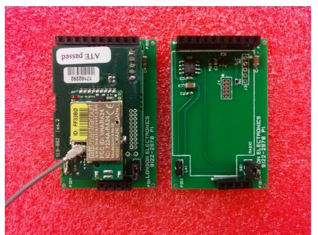
Left. Attached Radio I/F Module to handler board.
