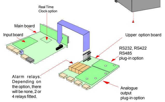
The analogue output and RS232 or RS422 plug-in option boards are fixed to the upper option board with white plastic pillars. You must apply a firm force when fitting or removing these options.
