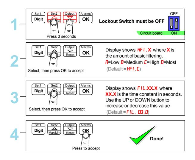
See also Filter Jump setting in the Advanced Menu, if your signal is particularly noisy and you cannot get sufficient smoothing with this filter.
