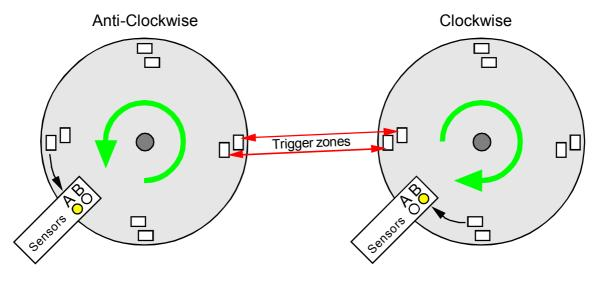
Sensor A triggers before sensor B
