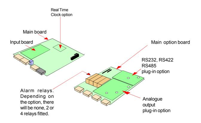
The analogue output and RS232 or RS422 plug-in option boards are fixed to the main option board with white plastic pillars. You must apply a firm force when fitting or removing these options.
