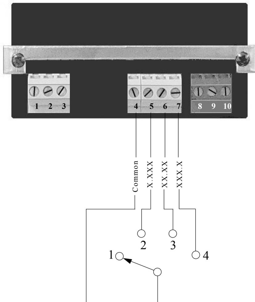
In the example shown, a 4 way rotary switch allows 4 decimal point choices to be selected, 1] XXXX 2] X.XXX 3] XX.XX 4] XXX.X
