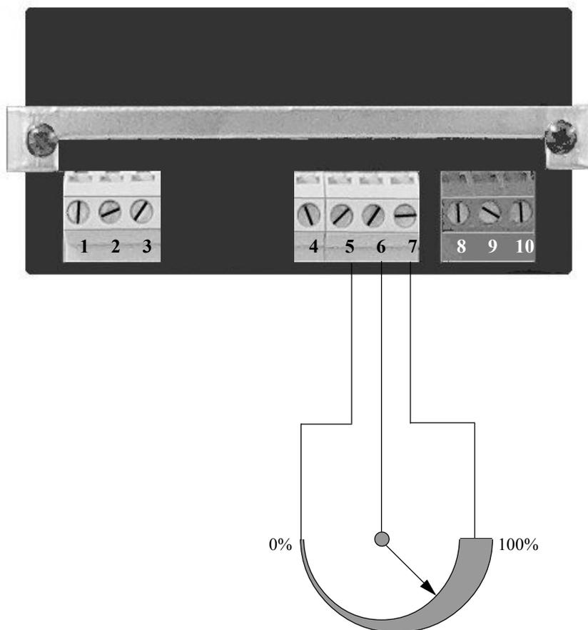
In the example shown, a 1Kilohm linear potentiometer allows adjustment from 0% to 100 % brightness.
