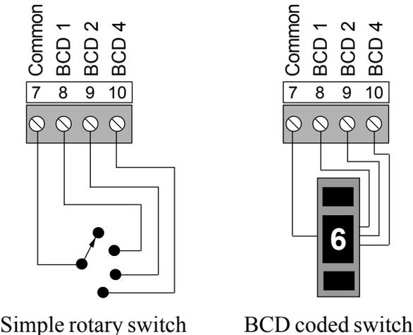
If you wish to use a rotary switch to select up to 8 memory locations, and to switch up to 8 two-wire signals, we make a 1/8 DIN rotary switch model SW2P8W-BCD for this purpose.
