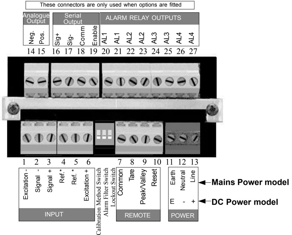
**NB - Switches have changed! Red switches had ON=UP. Blue switches have ON=DOWN**
