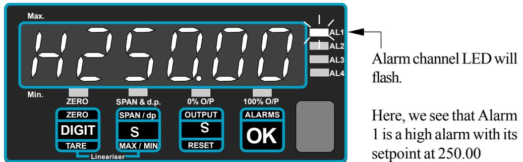
To change alarm settings, select the alarm you wish to change as shown above until its LED is flashing, then press the ALARM key for more than 3 seconds. You will see one digit is brighter than the others. You can change its value using the UP/DOWN buttons, and then select other digits with the DIGIT SELECT pushbutton.
