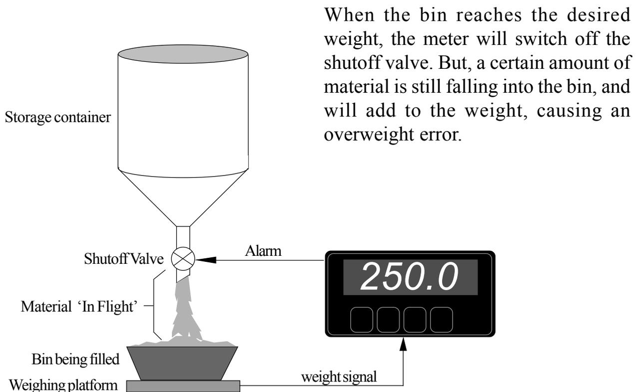
When the bin reaches the desired weight, the meter will switch off the shutoff valve. But, a certain amount of material is still falling into the bin, and will add to the weight, causing an overweight error.
