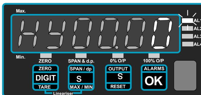
The hysteresis value is directly related to your measurements, so, for example, if you have a high alarm, set to 500, and set the hysteresis value to 7, the alarm will occur when the meter reading rises above 500, and will reset when the meter reading falls to 493. If the hysteresis is set to 9999, the alarms will be provided with 'IN-FLIGHT' compensation (automatic correction for overshoot)
