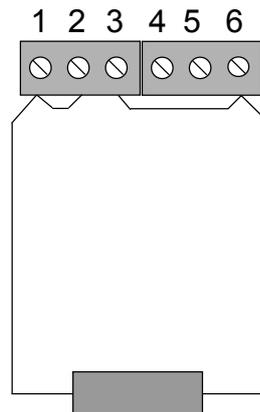
**2 wire connection (does not compensate for connector or cable resistance)**
