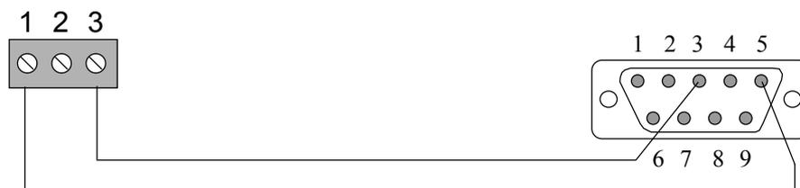
Interior view of a 9 pin D connector, which can be connected to a COM port connector on your PC.
