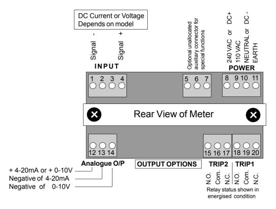
Please see appropriate section in this manual for connection details of BCD option or SERIAL output options. These options are mutually exclusive, and are not available with Analogue output or Trip output options.
