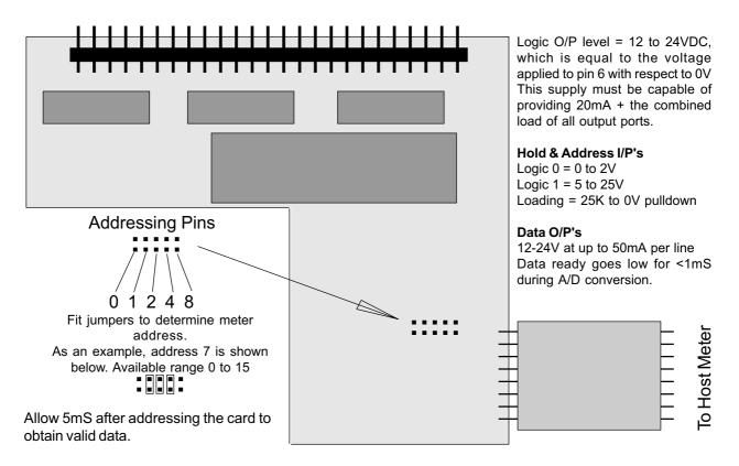
This option derives its data directly from the meter's A/D convertor. This data is updated every 400 milliseconds, but can be accessed within 5 milliseconds. The outputs and handshake lines are fully isolated from the meter to a level of 380 VAC. The option must be powered externally, typically from your PLC accessory supply.
