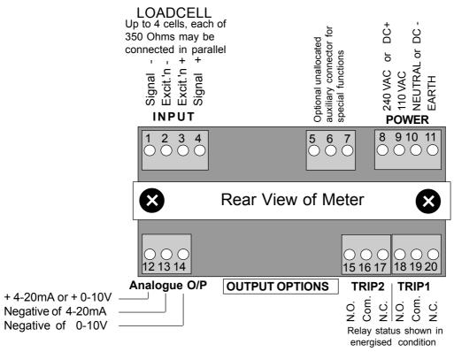
Please see appropriate section in this manual for connection details of BCD option or SERIAL output options. These options are mutually exclusive, and are not available with Analogue output or Trip output options.
