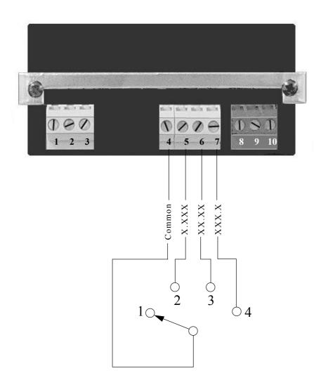
In the example shown, a 4 way rotary switch allows 4 decimal point choices to be selected, 1] XXXX 2] X.XXX 3] XX.XX 4] XXX.X
