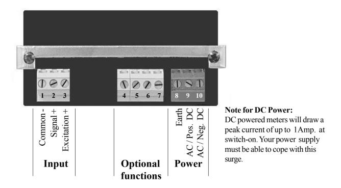
Use screened cable for your input signal and connect the screen to power earth at the meter end of the cable only. For best performance, keep the signal cable well away from power cables, which could carry electrical noise likely to interfere with your measurement.
