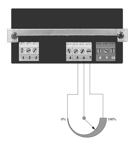
In this example, a 1Kilohm linear potentiomer allows adjustment from 0% to 100 % brightness.
