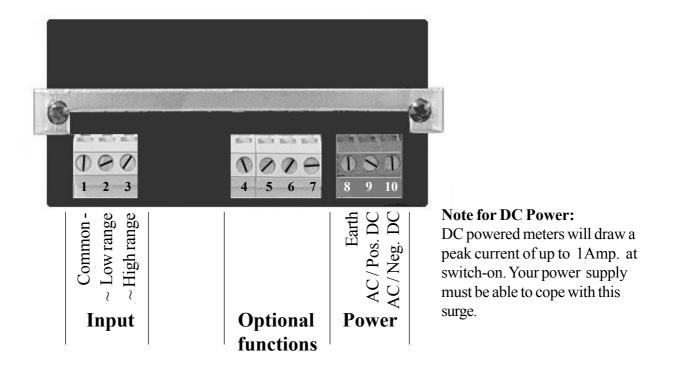
Use screened cable for your input signal and connect the screen to power earth at the meter end of the cable only. For best performance, keep the signal cable well away from power cables, which could interfere with your measurement.
