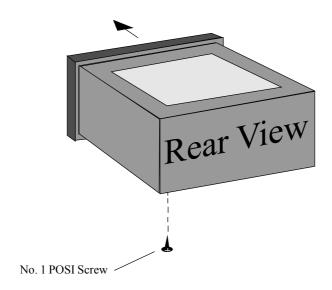
Withdraw the whole assembly from the front. Cut and solder links in new position, as required, and replace assembly, screw and front cover.
