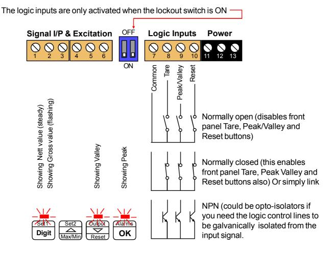
To enable the front panel buttons, you must connect the logic input for that function to common. If you want to have both front panel and remote tare, reset and peak/valley functions, you can use normally closed pushbuttons for the remote switches.
