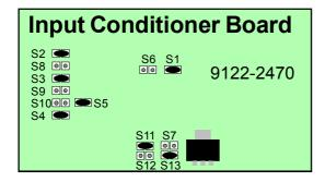
**Default Input configuration switches** Link S1, S2, S3, S4, S5, S11, S13. Open S6, S7,S8, S9, S10, S12
