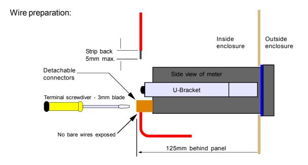
We recommend multi-strand wire, because it withstands vibration better than single strand cable. Pull the wire firmly after you make the connection to confirm it is tight.
