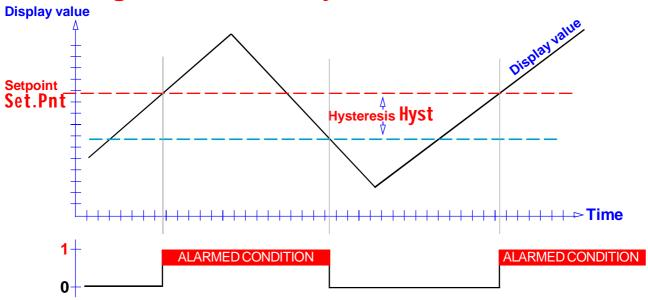
The Setpoint can be placed anywhere you like, in the range **!99999** to **+999999** and will include a decimal point in the appropriate position if you have set your display range to have a decimal point.
