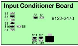
**Default Input configuration switches** Link S8, S9, S10, S11. Open S2, S3, S4, S12
