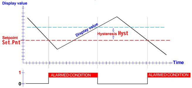
The Setpoint can be placed anywhere you like, in the range **!99999** to **+999999** and will include a decimal point in the appropriate position if you have set your display range to have a decimal point.
