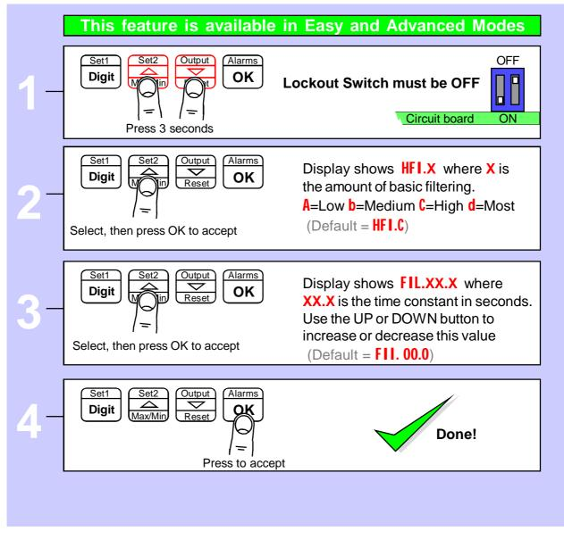
See also Filter Jump setting in the Advanced Menu, if your signal is particularly noisy and you cannot get sufficient smoothing with this filter.
