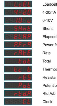
4-20mA Elapsed timer Power frequency Thermocouples Resistance Potentiometer Rtd.A/b
