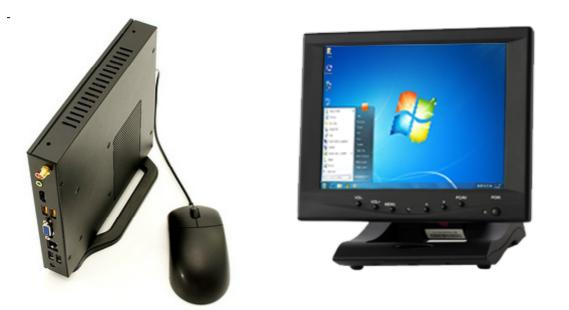
These miniature PCs can be used to collect data from our LineLogger modules and publish the data live to the web, or they can be used to allow operators to select downtime or fault reasons from a list, so that a history of reasons can be created in real time.
