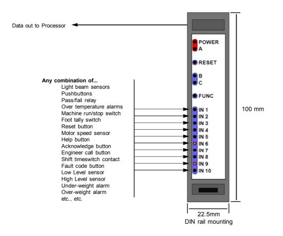
Each LineLogger (you can have up to 32 of them) can accept up to 10 inputs, which could be ...
