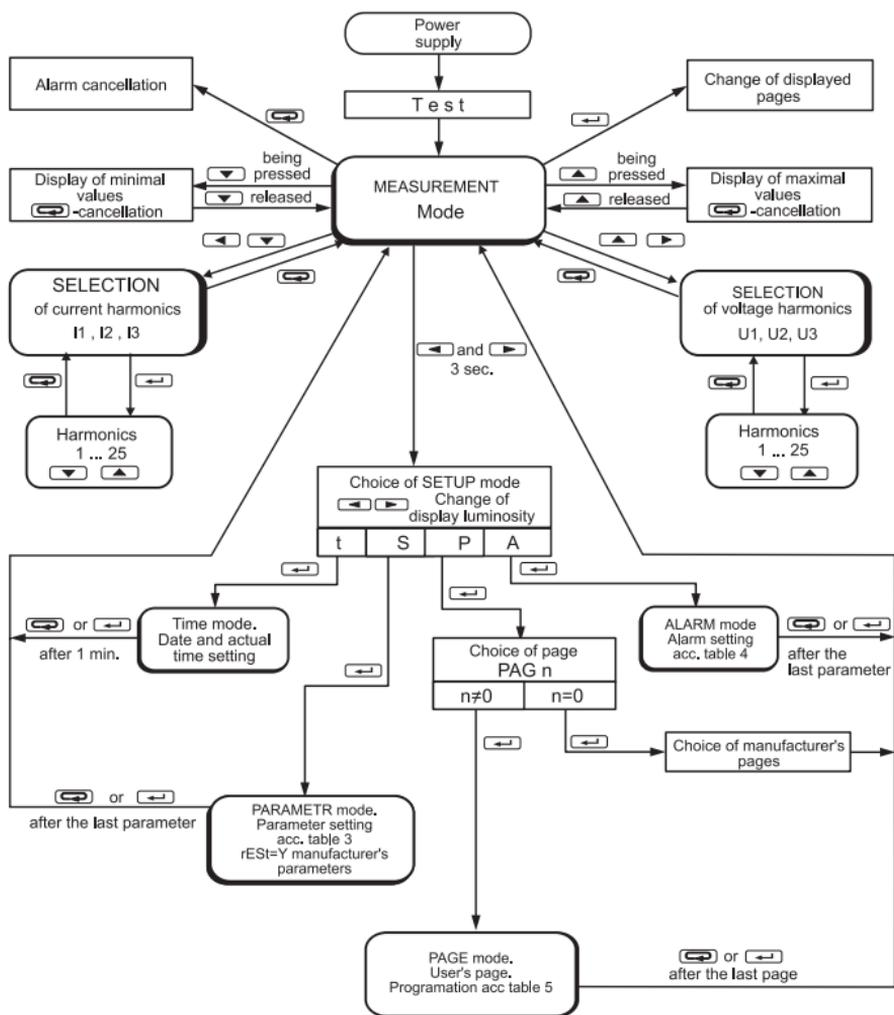
**Fig.6 N10 meter working modes.**
