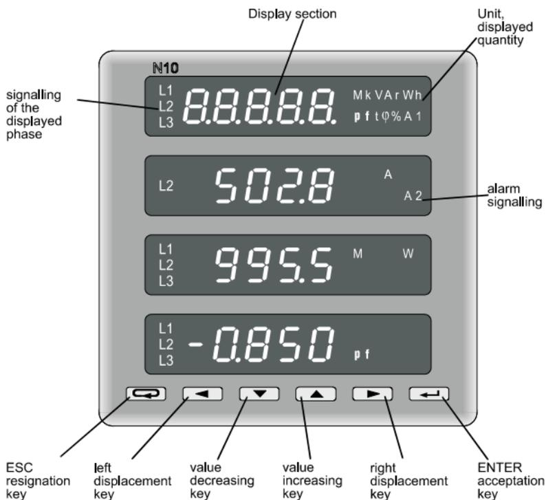
**Fig. 5. View of the N10 meter faceplate**
