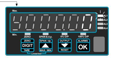
The hysteresis value is directly related to your measurements, so, for example, if you have a high alarm, set to 500, and set the hysteresis value to 7, the alarm will occur when the meter reading reaches 500, and will reset when the meter reading falls to 493.
