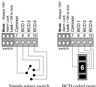
If you want to use a rotary switch to select up to 8 memory locations, and to switch up to 8 two-wire signals, switch model SW2P8W-BCD may be useful. This is a 1/8DIN unit you can order separately.
