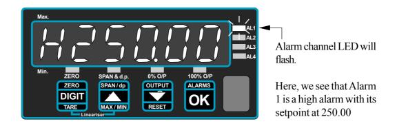
To change alarm settings, choose an alarm as shown above, then press the ALARM key for more than 3 seconds. You will see one digit brighter than the others. You can change its value using the UP/DOWN buttons. Select other digits with the DIGIT SELECT pushbutton.
