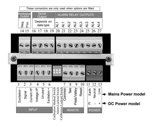
Cabling should be screened and routed away from noise-carrying cables and machines to reduce interference. The screen can be connected to power earth if it is not already grounded at the sensor end.
