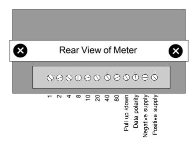
Pullup/pulldown: Connect this terminal to Negative supply to pull down the input signal if using PNP
