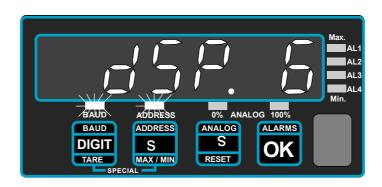
After you press the OK button after the Data edit 'LOSE' setting, the display will show 'dSP.3' or 'dSP.4' or 'dSP.5' or 'dSP.6' (dSP means 'display')
