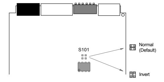
Refit the board into the case, replace the small retaining screw and re-install.
