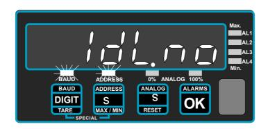
'IdL. 10' means the display will show the last received data permanently. 'IdL. 3' means the display will show ----- if no data arrives for 3 seconds 'IdL. 10' means the display will show ----- if no data arrives for 10 seconds 'IdL. 30' means the display will show ----- if no data arrives for 30 seconds 'IdL. 60' means the display will show ----- if no data arrives for 60 seconds
