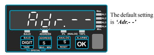
To change the address, use the UP/DOWN buttons. Press OK when you've selected the correct address.
