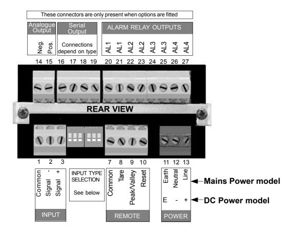
Input and contact-closure remote cabling should be screened and routed away from noise-carrying cables to prevent spurious interference.
