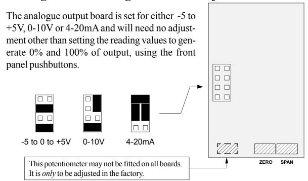
To change a range, for example from 0-10V to 4-20mA, you must reposition some jumpers as shown above, and adjust the zero and span potentiometers to get the correct output levels at 0% and 100%. Look on the top and bottom surfaces of the case, near the rear. You will see two small screws, one on each surface.
