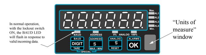
All programming adjustments are made via the front panel pushbuttons, which use LED annunciators to show which setting is being altered at any time. A clear protective window is provided, behind which you can fit one of our 'Units-of-Measure' labels, to identify the reading as Kg, or Deg. C, or Bar, etc.
