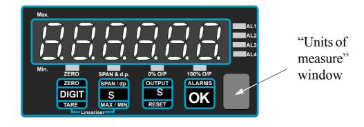
The front panel pushbuttons each have an LED to show which setting is being altered at any time. A clear protective window is provided, behind which you can fit one of our 'Units-of-Measure' labels, normally the OHM symbol
