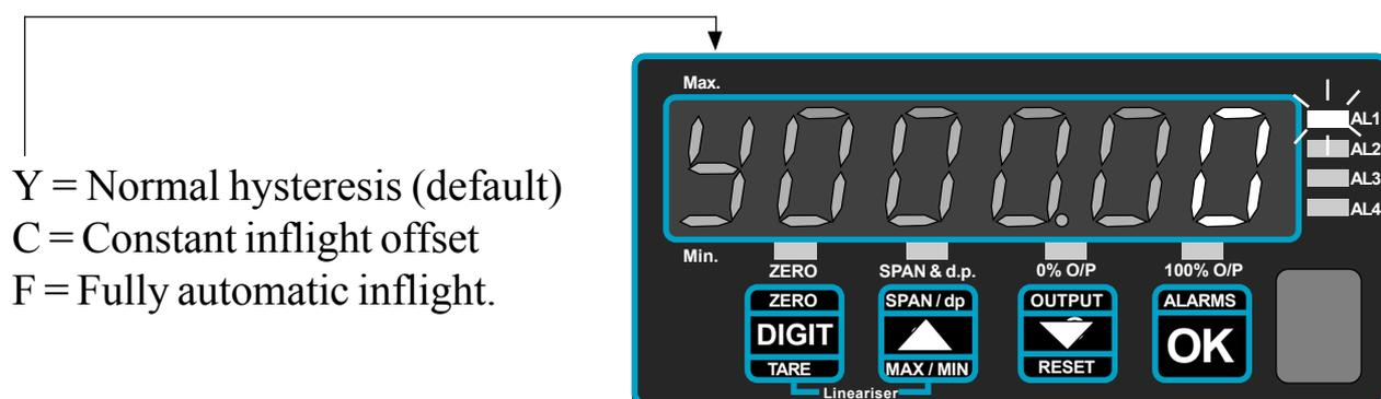
The hysteresis value is directly related to your measurements, so, for example, if you have a high alarm, set to 500, and set the hysteresis value to 7, the alarm will occur when the meter reading reaches 500, and will reset when the meter reading falls to 493.
