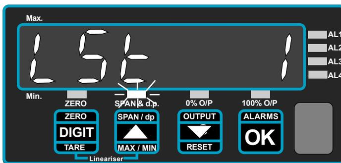
Use the UP/DOWN buttons to select a roundup value, and accept by pressing OK.
