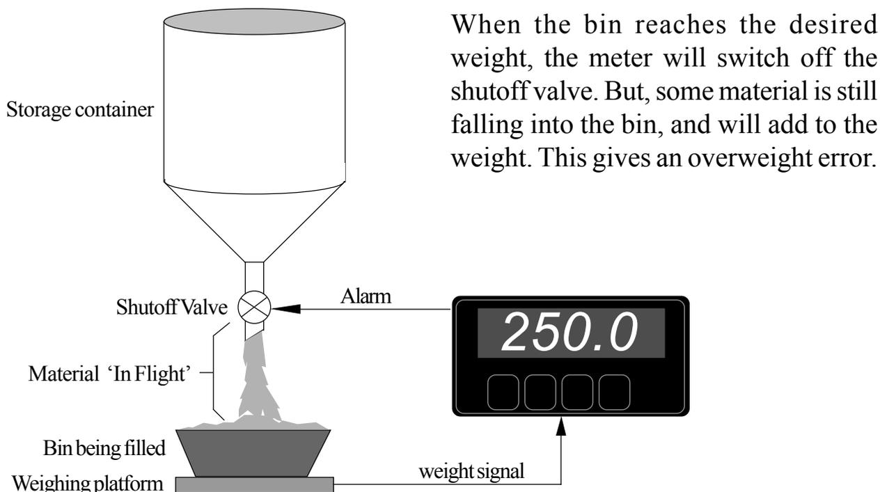
When the bin reaches the desired weight, the meter will switch off the shutoff valve. But, some material is still falling into the bin, and will add to the weight. This gives an overweight error.
