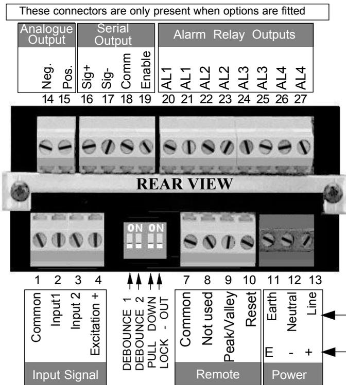
The ON position is marked on the switch and may differ with different manufacturers.
