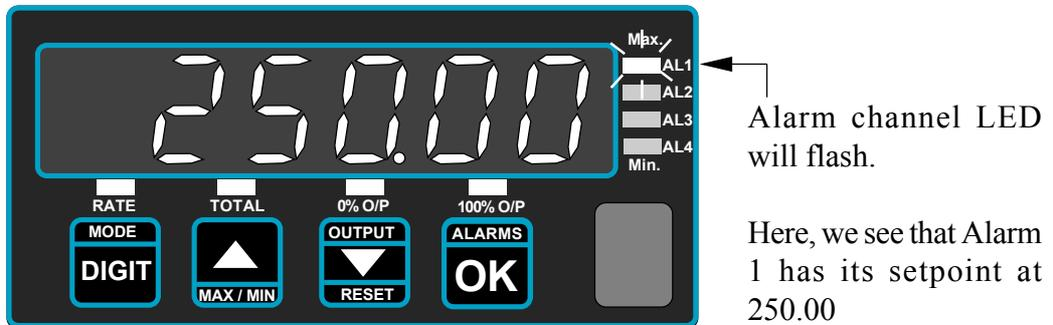
To change alarm settings, select the alarm you wish to change as shown above until its LED is flashing, then press the ALARM key for more than 3 seconds. You will see one digit is brighter than the others. You can change its value using the UP/DOWN buttons, and then select other digits with the DIGIT SELECT pushbutton. When the value has been set, press OK.
