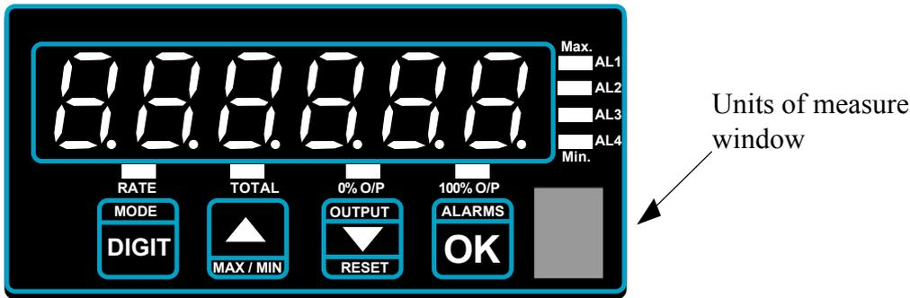
To change variables when the meter is unlocked, select digits using the DIGIT key, and increase or decrease with UP and DOWN key. When the setting is correct, press OK.
