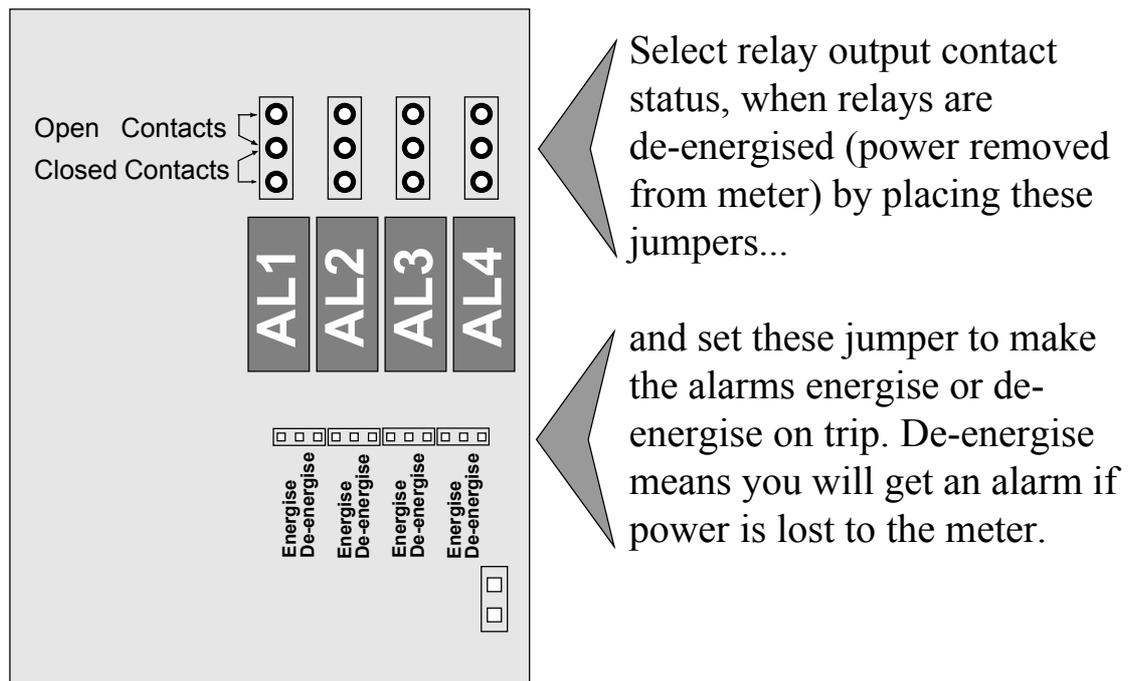
When you have set the jumpers, refit the board to the meter and carefully slide the assembly back into the case.
