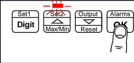
Apply the highest calibration signal you can achieve, ideally 100% of system capacity. You can use less, but you will get better accuracy with higher signals. Now press OK
