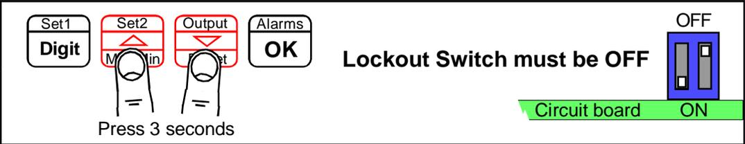
Lockout Switch must be OFF
