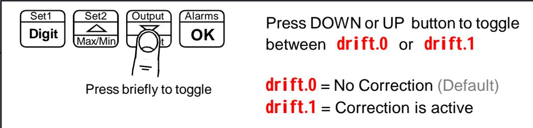
Press DOWN or UP button to toggle between **drift.0** or **drift.1**
