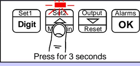
Press Set2 for 3 seconds. You can now set your decimal point position using the UP or DOWN buttons. Press OK when done.
