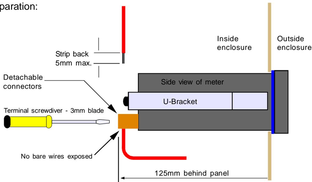
We recommend multi-strand wire, because it withstands vibration better than single strand cable. Pull the wire firmly after you make the connection to confirm it is tight.
