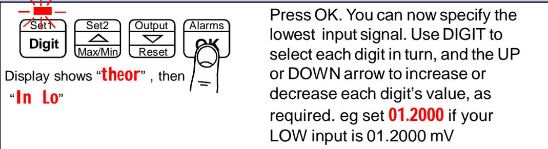
Press OK. You can now specify the lowest input signal. Use DIGIT to select each digit in turn, and the UP or DOWN arrow to increase or decrease each digit's value, as required. eg set **01.2000** if your LOW input is 01.2000 mV
