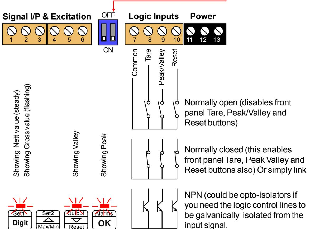
To enable the front panel buttons, you must connect the logic input for that function to common. If you want to have both front panel and remote tare, reset and peak/valley functions, you can use normally closed pushbuttons for the remote switches.
