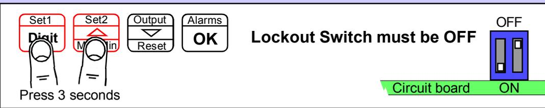
**Lockout Switch must be OFF**
