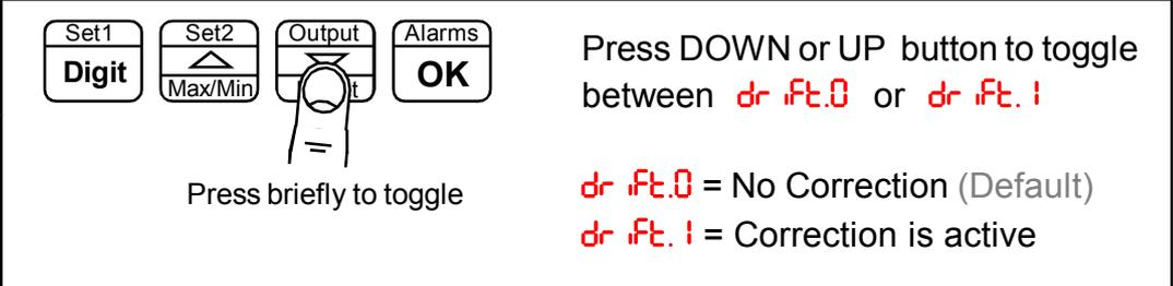
Press DOWN or UP button to toggle between **drift.0** or **drift.!**
