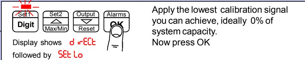
Apply the lowest calibration signal you can achieve, ideally 0% of system capacity. Now press OK
