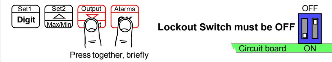
Lockout Switch must be OFF
