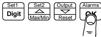
Display shows each of the parameters and you can move on to the next one with the OK button.
