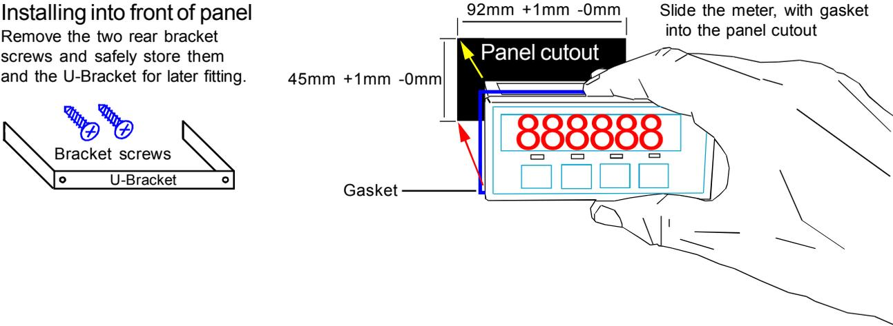
Slide the meter, with gasket into the panel cutout
