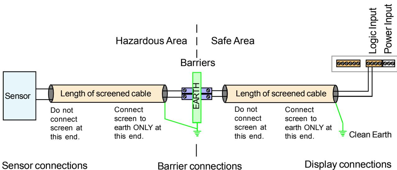
When using multi-core screened cable to connect several displays to several sensors, please be sure to use one twisted pair for each display and sensor.
