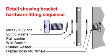
The side holes in the two brackets are 8.5mm dia. to accept M8 bolts.
