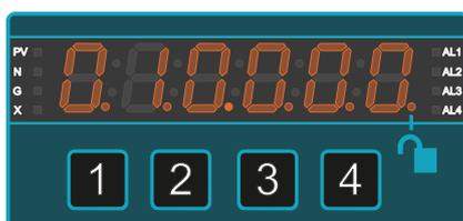
To set decimal point position, press button **2** (Cal Hi) for 3 seconds and move the decimal point to the desired position with buttons **2**( $\Delta$ ) or **3**( $\nabla$ ) .Press button **4** (OK) to save.
