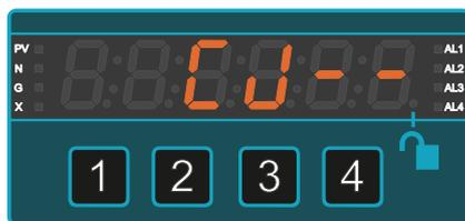
To set a fixed cold junction temperature press buttons **2** ( $\Delta$ ) or **3** ( $\nabla$ ) to change the display to show **'CJ - -'**
