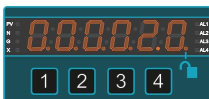
To set decimal point position, press button **2** (Cal Hi) again for 3 seconds and move the decimal point to the desired position with buttons **2** ( $\Delta$ ) or **3** ( $\nabla$ ) .
