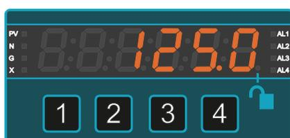
Apply 50% of input range, so 125 A in the example and ensure the display reads 50% of display range, being 125.0 in the example.
