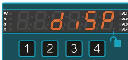
Press and hold buttons **3** and **4** together for at least 3 seconds until the display shows 'diSP'.
