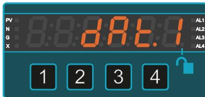
Press and hold buttons **2** ( $\Delta$ ) and **4** (OK) together for at least 6 seconds.
