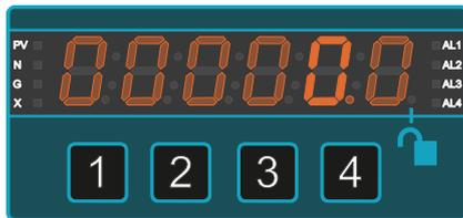
Press buttons **2** ( $\Delta$ ) or **3** ( $\nabla$ ) buttons to set 0.0 or your desired 'rdLo' reading.
