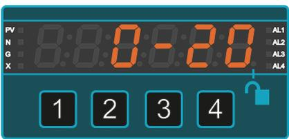
Press and hold button 3 (▽) for 3 seconds until the display shows what option is installed, either '0-20', '4-20' or '0-10'.
