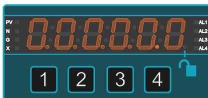
To set decimal point position, press button **2** (Cal Hi) for 3 seconds and move the decimal point to the desired position with buttons **2** ( $\Delta$ ) or **3** ( $\nabla$ ).
