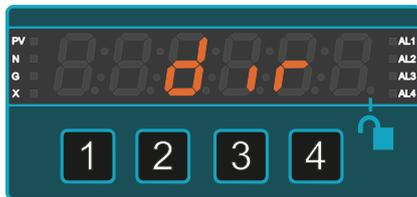
8 Apply the highest load value, ideally 100% of full load, and press button **4** (OK).
