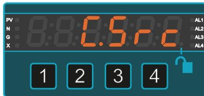
Press button **1** and **2** together for 3 seconds until you see 'C.Src' (calibration source)
