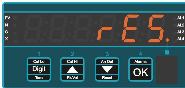
Resistance mode is ideal for measuring and checking the resistance of components such as inductors, heaters, transformers and earth bonds.
