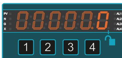
Press button **1** (Digit) to select each digit and edit with buttons **2** ( $\Delta$ ) or **3** ( $\nabla$ ) to show 0.0 or your desired low reading.Press button **4** (OK) when all digits are correct.
