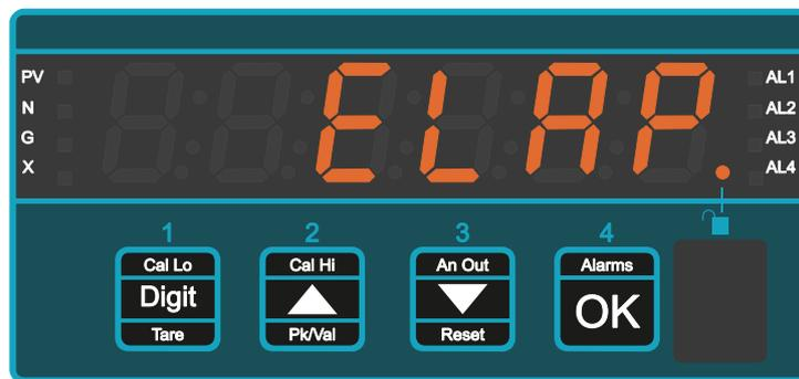
Elapsed timer mode is ideal for a wide range of applications, such as process timing, takt timing, countdown to completion etc.
