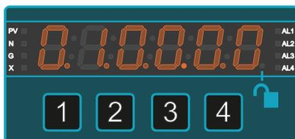
11 Press button **1** (Digit) to select each digit and edit with buttons **2** ( $\Delta$ ) or **3** ( $\nabla$ ) to show your desired high reading.
