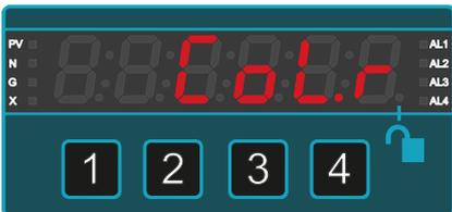
Press and hold buttons **3** and **4** together for at least 3 seconds.
