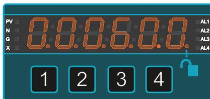
To set decimal point position, press and hold button **2** (Cal Hi) again for 3 seconds and move the decimal point to the desired position with buttons **2** ( $\Delta$ ) or **3** ( $\nabla$ ).Press button **4** (OK) to save.
