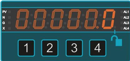
Press button 1 (Digit) to select each digit and edit with buttons 2 ( $\Delta$ ) or 3 ( $\nabla$ ) buttons to show your desired low reading.
