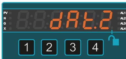
If there are 2 data ports installed, you can now press the button **2** ( $\Delta$ ) or **3** ( $\nabla$ ) to select Channel 2, '**dAt.2**'
