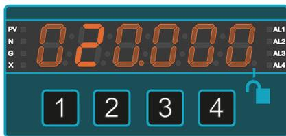
Press button **1** (Digit) to select each digit and edit with buttons **2** ( $\Delta$ ) or **3** ( $\nabla$ ) to show 20.000 or your desired high reading.Press button **4** (OK) when all digits are correct.
