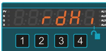
10 To set decimal point position, press button **2** (Cal Hi) again for 3 seconds and move the decimal point to the desired position with buttons **2** ( $\Delta$ ) or **3** ( $\nabla$ ).
