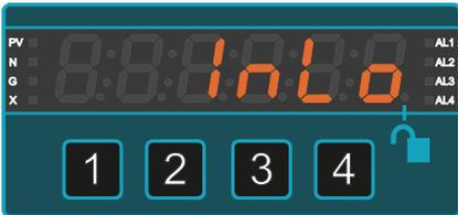
Apply the lowest load value, usually 0kg, to your load cell, and press button 4 (OK).
