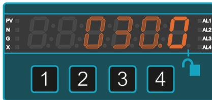
Press button **1** (Digit) to select each digit and edit with button **2** ( $\Delta$ ) or **3** ( $\nabla$ ) to define how often you will check for drift, in seconds.
