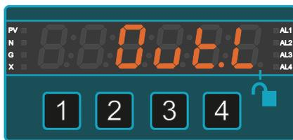
'Out.L' will appear, prompting you to set the measurement which generates the minimum analogue output signal. For example 4mA.
