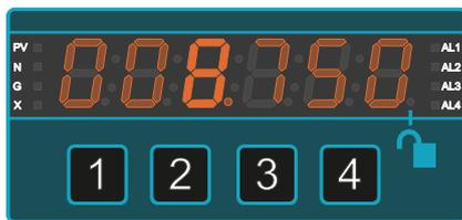
Press button **1** (Digit) to select each digit and edit with buttons **2** ( $\Delta$ ) or **3** ( $\nabla$ ) to show 8.750 or your desired high reading.
