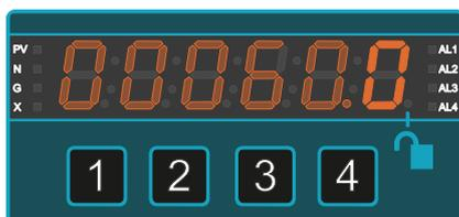
Press button **1** (Digit) to select each digit and edit with buttons **2** ( $\Delta$ ) or **3** ( $\nabla$ ) to show 60.0 or your desired high reading.Press button **4** (OK) when all digits are correct.
