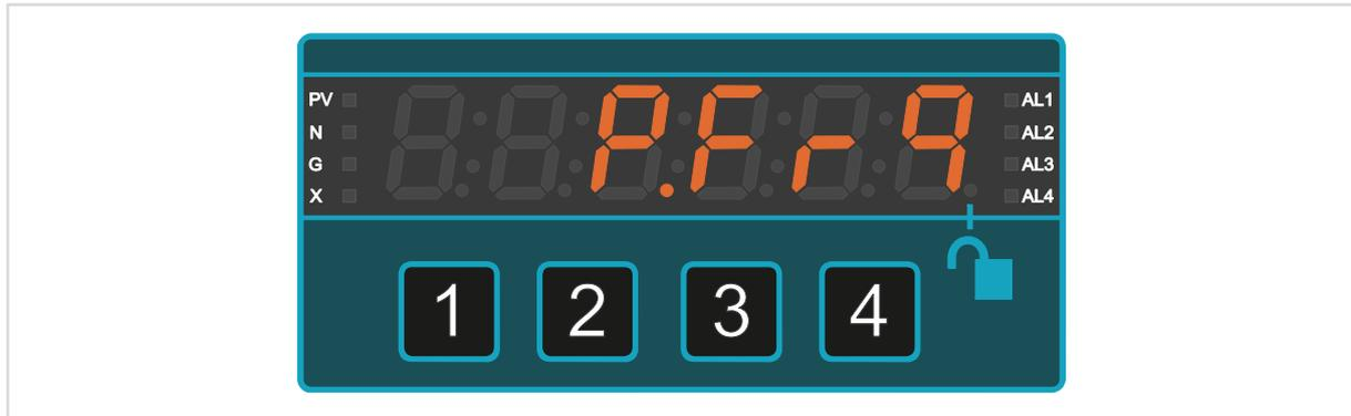
Range 47.000 to 63.000 Hz. 95-265V AC. The meter measures the frequency of its own power voltage, no auxiliary connection is needed.
