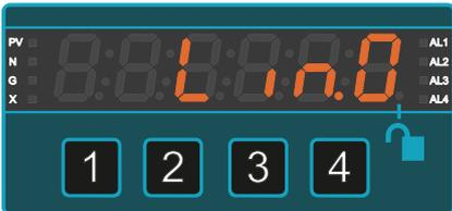
Press and hold buttons **2** and **3** together for at least 3 seconds until the display shows 'Lin.0' or 'Lin.1'
