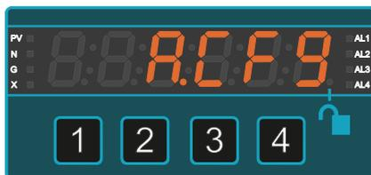
Press and hold the button 1 (OK) for at least 6 seconds until you see 'A.CFG'
