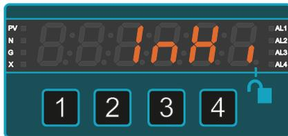
Apply the high level calibration signal 9.000V in the example, and press button **4** (OK).
