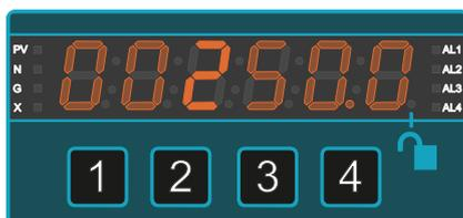
Press button **1** (Digit) to select each digit and edit with buttons **2** ( $\Delta$ ) or **3** ( $\nabla$ ) to show 250.0 or your desired high reading.
