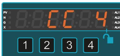
To choose which contact closure channel to view or edit press button **2**( $\Delta$ ) or **3**( $\nabla$ ) button to select a channel.
