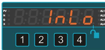
Apply the low level calibration signal 1.000V in the example, and press button **4** (OK).
