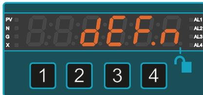
Press and hold buttons **1**, **2**, **3** and **4** together for at least 3 seconds until the display shows 'dEF.n' (Defaults no).
