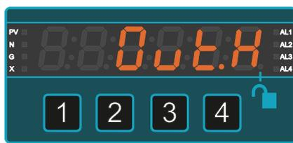
'Out.h' will appear, prompting you to set the measurement which generates the maximum analogue output signal. For example 20mA.
