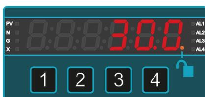
Apply 50% of input range, so 5.000V in the example and ensure the display reads 50% of display range, being 30.0 in the example.
