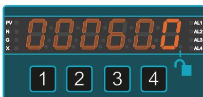
Press button **1** (Digit) to select each digit and edit with buttons **2** ( $\Delta$ ) or **3** ( $\nabla$ ) to show 60.0 or your desired high reading.
