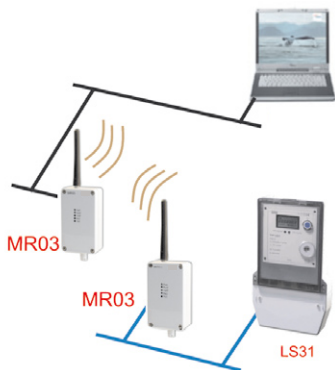
Fig 1. Exemplary remote readout of LS31 watt-hour using the MR03 module
